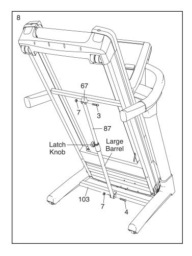
With the help of a second person, raise the front of the treadmill and insert the crossbar on the Base (103) into the cutout in the cardboard stand as shown. Have the second person hold the treadmill to prevent it from moving forward or backward.
